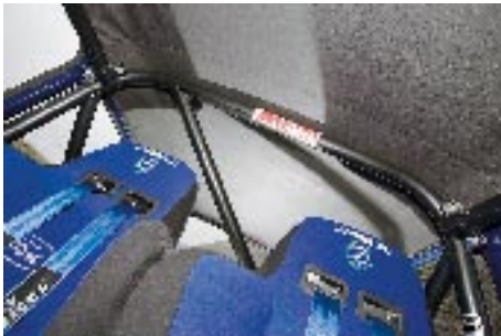
Safety Devices cage gives the Anglia some motorsport muscle, plus it's a must when Wayne gives the Zetec lump some abuse.
